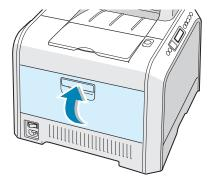
If you have installed the toner cartridges incorrectly, the left cover will not close properly. Check again to make sure the cartridge colors correspond to those marked on the right hand side. Never use force to close the cover.
